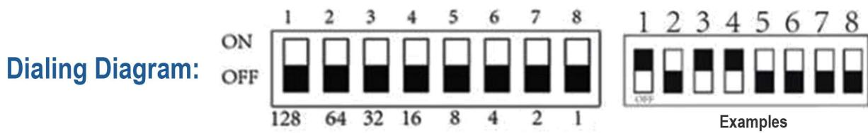
Note: The above picture is a schematic diagram of the DIP switch. The DIP switch has 8 DIP positions. The corresponding numbers from 1 to 8 are 128, 64, 32, 16, 8, 4, 2, 1, and these values are added together as the address code. As shown in the figure above, bits 1, 3, and 4 are in the ON position, so the address code is  $128+32+16=176$ , that is, the address code is 176
